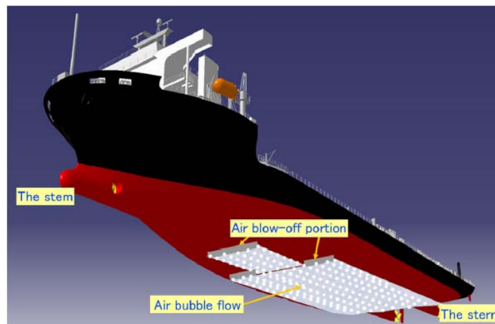
Fig 4 Air Bubbles discharged below the actual Hull
